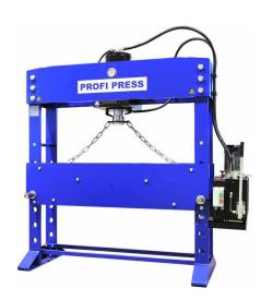
This 100-ton Workshop Press has a working width of 1500 mm and a 380 mm stroke and can be operated with a joystick or handpump and has 2 speeds controlled with an easy to use lever directly on the hydraulic control unit. A pressure regulation gauge is clearly displayed on the front of the machine for easy control of pressing operations.
