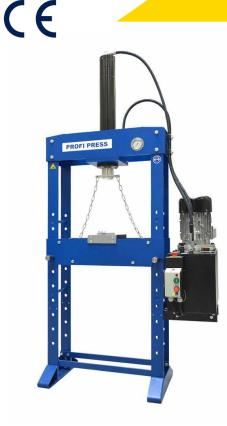
This broaching press from Profi Press is exclusively made in the Netherlands and has a capacity of 15 tons. The piston stroke is 600 mm and the hydraulic press includes a hand operated up/down valve for the movement of the piston, a pressure control valve and a speed control valve.
