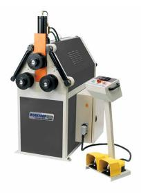
The PBH-45 Profile bender has 45 mm shafts 3 driven rolls driven either by a or a 3-Phase motor and comes with a standard set of section rolls that are configurable and are suitable for most bending applications of square or angular profiles. If you wish to bend round tubes or pipe, we have tools ready to go off the shelf for all common sizes such as 42.2 mm and 48.3 mm outside diameters along with many other sizes being readily available. If you are wanting to bend custom profiles all we need
