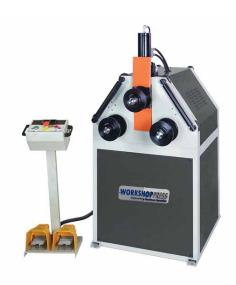
The PBH-50-2 Profile bender has 50 mm shafts and 2 driven bottom rolls driven either by a 1-Phase or a 3-Phase motor and comes with a standard set of section rolls that are configurable and are suitable for most bending applications of square or angular profiles. If you wish to bend round tubes or pipe, we have tools ready to go off the shelf for all common sizes such as 42.2 mm and 48.3 mm outside diameters along with many other sizes being readily available. If you are wanting to bend custom
