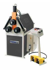
The PBH-55 Profile bender has 55 mm shafts 3 driven rolls driven either by a or a 3-Phase motor and comes with a standard set of section rolls that are configurable and are suitable for most bending applications of square or angular profiles. If you wish to bend round tubes or pipe, we have tools ready to go off the shelf for all common sizes such as 42.2 mm and 48.3 mm outside diameters along with many other sizes being readily available. If you are wanting to bend custom profiles all we need
