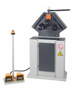
The PBM-30 Profile bender has 30 mm shafts and 2 driven bottom rolls driven either by a 1-Phase or a 3-Phase motor and comes with a standard set of section rolls that are configurable and are suitable for most bending applications of square or angular profiles. If you wish to bend round tubes or pipe, we have tools ready to go off the shelf for all common sizes such as 42.2 mm and 48.3 mm outside diameters along with many other sizes being readily available. If you are wanting to bend custom
