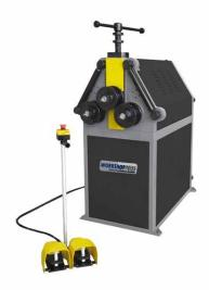
The PBM-45 Profile bender has 45 mm shafts and 3 driven rolls driven either by a 1-Phase or a 3-Phase motor and comes with a standard set of section rolls that are configurable and are suitable for most bending applications of square or angular profiles. If you wish to bend round tubes or pipe, we have tools ready to go off the shelf for all common sizes such as 42.2 mm and 48.3 mm outside diameters along with many other sizes being readily available. If you are wanting to bend custom
