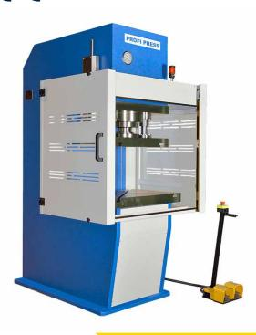
This 100-ton C-frame by RHTC Profi Press is suitable for performing work involving deep-drawing, forming and stamping, riveting, and many other applications. It has a throat depth of 325 mm and a working speed of 6.2 mm/s which is preluded by and an approach speed of 31 mm/s. After the cycle is completed the top plate returns at a rate of 48 mm/s. Maximum stroke of the top plate is 250 mm with the press having an overall shut height of 400 mm.
