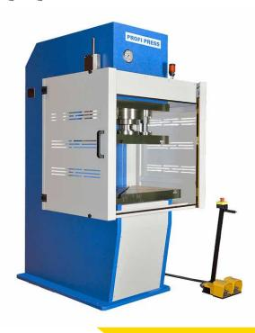
This 150-ton C-frame by RHTC Profi Press is suitable for performing work involving deep-drawing, forming and stamping, riveting, and many other applications. It has a throat depth of 375 mm and a working speed of 4 mm/s which is preluded by and an approach speed of 20 mm/s. After the cycle is completed the top plate returns at a rate of 31 mm/s. Maximum stroke of the top plate is 250 mm with the press having an overall shut height of 400 mm.
