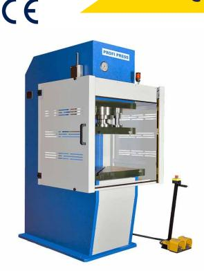
This 50-ton C-frame by RHTC Profi Press is suitable for performing work involving deep-drawing, forming and stamping, riveting, and many other applications. It has a throat depth of 265 mm and a working speed of 6.3 mm/s which is preluded by and an approach speed of 32 mm/s. After the cycle is completed the top plate returns at a rate of 42 mm/s. Maximum stroke of the top plate is 250 mm with the press having an overall shut height of 400 mm.
