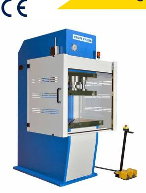
This 80-ton C-frame by RHTC Profi Press is suitable for performing work involving deep-drawing, forming and stamping, riveting, and many other applications. It has a throat depth of 290 mm and a working speed of 6 mm/s which is preluded by and an approach speed of 25 mm/s. After the cycle is completed the top plate returns at a rate of 36 mm/s. Maximum stroke of the top plate is 250 mm with the press having an overall shut height of 400 mm.
