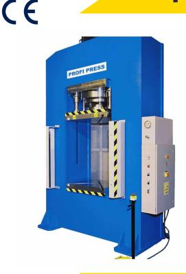
The RHTC Profi Press also offers high-quality hydraulic production presses like the PPRM-100. This heavy-duty production 100-ton production press is suitable for stamping, die-cutting, deep-drawing and forming. The frame of this press is made from S355JR steel and is electro-welded to assure a solid press framework that will last a lifetime which is demonstrated by the presses massive weight of 2340 Kg. This machine comes with 2 speeds and an integrated pressure manometer.
