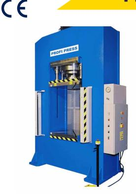
The RHTC Profi Press also offers high-quality hydraulic production presses like the PPRM-220. This heavy-duty production 220-ton production press is suitable for stamping, die-cutting, deep-drawing and forming. The frame of this press is made from S355JR steel and is electro-welded to assure a solid press framework that will last a lifetime which is demonstrated by the presses massive weight of 4680 Kg. This machine comes with 2 speeds and an integrated pressure manometer.
