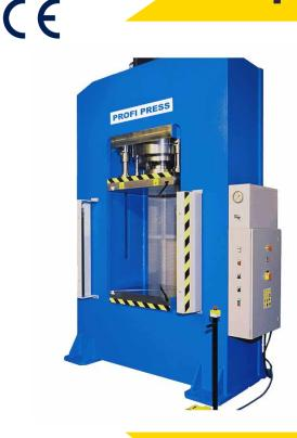
The RHTC Profi Press also offers high-quality hydraulic production presses like the PPRM-300. This heavy-duty production 300-ton production press is suitable for stamping, die-cutting, deep-drawing and forming. The frame of this press is made from S355JR steel and is electro-welded to assure a solid press framework that will last a lifetime which is demonstrated by the presses massive weight of 6490 Kg. This machine comes with 2 speeds and an integrated pressure manometer.
