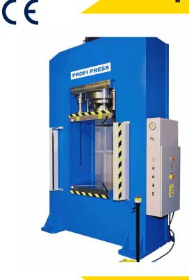
The RHTC Profi Press also offers high-quality hydraulic production presses like the PPRM-500. This heavy-duty production 500-ton production press is suitable for stamping, die-cutting, deep-drawing and forming. The frame of this press is made from S355JR steel and is electro-welded to assure a solid press framework that will last a lifetime which is demonstrated by the presses massive weight of 12150 Kg. This machine comes with 2 speeds and an integrated pressure manometer.aa
