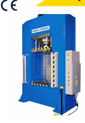
The RHTC Profi Press also offers high-quality hydraulic production presses like the PPRM-80. This heavy-duty production 80-ton production press is suitable for stamping, die-cutting, deep-drawing and forming. The frame of this press is made from \$355JR steel and is electro-welded to assure a solid press framework that will last a lifetime which is demonstrated by the presses massive weight of 2080 Kg. This machine comes with 2 speeds and an integrated pressure manometer.
