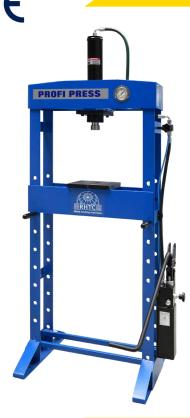
This 15-ton Workshop Press has a working width of 560 mm and a 160 mm stroke and can be operated with by hand or by foot. A pressure regulation gauge is clearly displayed on the front of the machine for easy control of pressing operations.
