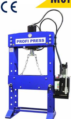
This **30-ton Workshop Press** has a working width of 750 mm and a 380 mm stroke and can be operated with a joystick or handpump and has 2 speeds controlled with an easy to use lever directly on the hydraulic control unit. A pressure regulation gauge is clearly displayed on the front of the machine for easy control of pressing operations.
