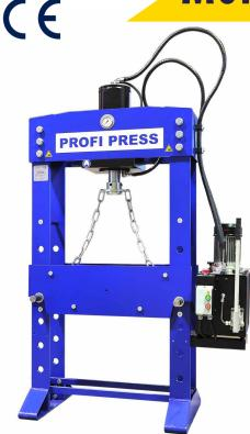
This 100-ton Workshop Press has a working width of 1100 mm and a 380 mm stroke and can be operated with a joystick or handpump and has 2 speeds controlled with an easy to use lever directly on the hydraulic control unit. A pressure regulation gauge is clearly displayed on the front of the machine for easy control of pressing operations.
