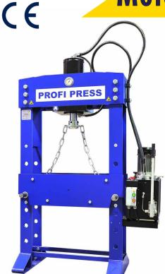
This **60-ton Workshop Press** has a working width of 750 mm and a 380 mm stroke and can be operated with a joystick or handpump and has 2 speeds controlled with an easy to use lever directly on the hydraulic control unit. A pressure regulation gauge is clearly displayed on the front of the machine for easy control of pressing operations.
