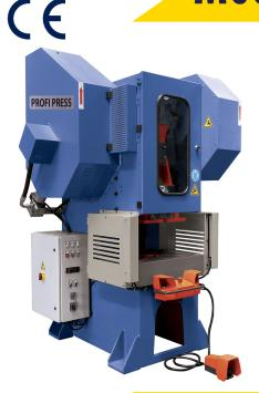
RHTC designed the Profi Press Mechanical C-frame presses for production work, and they are suitable for performing stamping, cutting and deep-drawing work. Profi Press Mechanical C-Frame Series Press are manufactured in Europe. RHTC produces the presses with nothing but high-quality components, made out of \$355JR steel and the quality is guaranteed. All presses are manufactured to EU Norms and are CE Certified.
