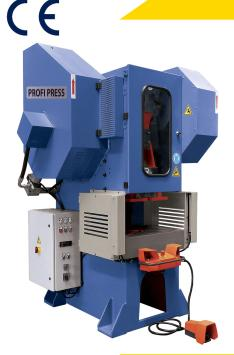
RHTC designed the Profi Press Mechanical C-frame presses for production work, and they are suitable for performing stamping, cutting and deep-drawing work. Profi Press Mechanical C-Frame Series Press are manufactured in Europe. RHTC produces the presses with nothing but high-quality components, made out of S355JR steel and the quality is guaranteed. All presses are manufactured to EU Norms and are CE Certified.
